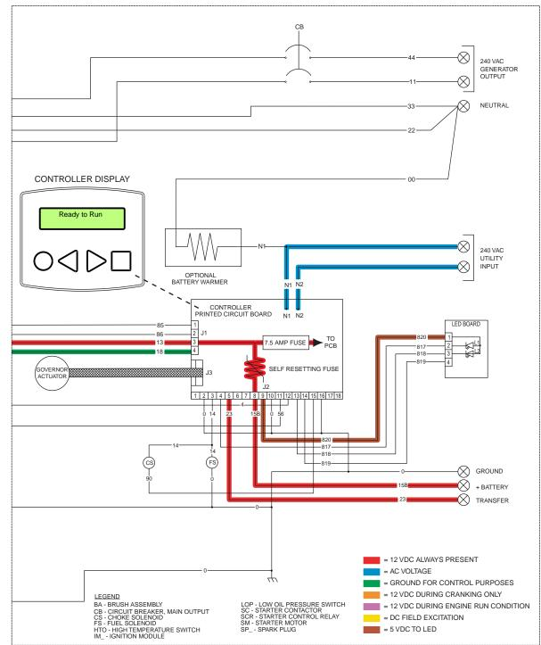
Figure 7. Circuit Condition - Retransfer to "Utility" and Engine Shutdown
